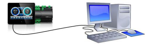
The network card of the computer must be configured in order to have the assignment of the DHCP address activated. In this case, the Vision Touch Wellness and the computer, finding no DHCP server, will take the default IP addresses previewed for the class of addressing 169.254.xxx.xxx. In order to connect to the device, it will be necessary to open up a browser page and digit in the address bar the following order:
