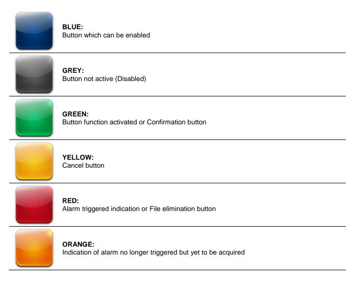
Some buttons have delayed activation to avoid unintentional commands (see standby for example). When pressed the progressive colour change is viewed until the function is activated.
