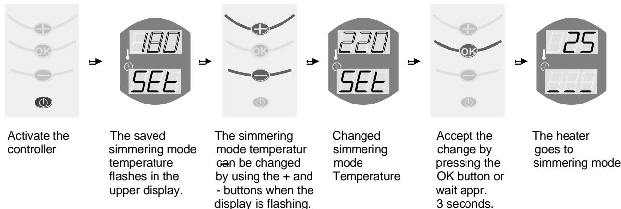
When the heater is on simmering mode, the lower led display indicates with dashed lines the simmering mode in relation to the requested temperature. The upper display indicates the current temperature of the stone space. The required simmering mode has been reached once all the three dashed lines are lit.
