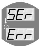
SEr Err (Serial Error) serial traffic error between the heater and the controller.
