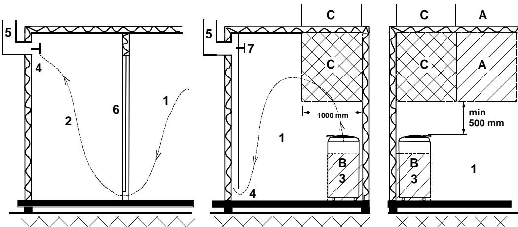
1. Sauna room                    3. Electric sauna heater                    5. Exhaust flue or channel
