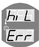
hiL Err (High Limit Error) stone space overheated (>400°C), electronic disconnection.
