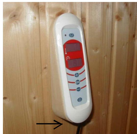
6. The frame is removed by pressing with a thin rod or a small screwdriver from the grooves (4) and turning carefully outwards.
